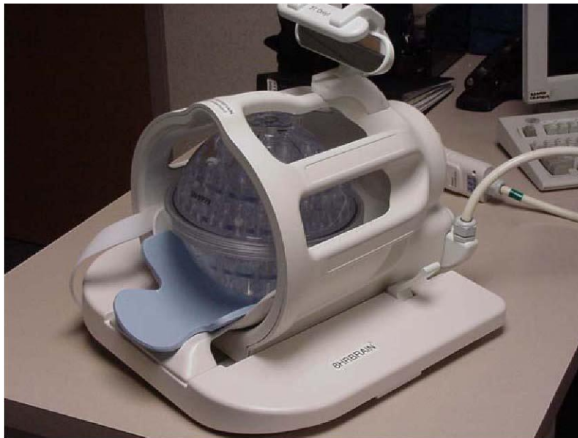
DIAN phantom shown positioned inside of an 8-channel head coil.
